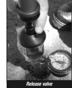
on the instrument for 10–15 seconds to allow air to rise and then release vacuum gently. Refill if necessary and replace cap until stopper comes in contact with bottom of the reservoir, then continue *tightening for 1/4 turn only*. Repeat pumping as above each time, after reading, for three or four times to improve sensitivity.
