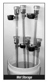
**Step 5 – Storage —** In seasonal cropping, where the ground will lie fallow over the winter, remove IRROMETERs *before* the first frost, clean exterior thoroughly with water. *DO NOT* let the
