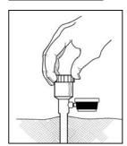
**Step 3 – Servicing —** Fill all IRROMETERS with a diluted solution of IRROMETER fluid (1 scant capful of concentrate to 1 gallon of water). Fill the IRROMETERS to the circle on the reservoir. Tap top of the IRROMETER with the palm of your hand to relieve any air lock. Take the vacuum pump and extract air from the instruments by pulling a vacuum of 80–85 cb (kPa) as registered on the gauge. Leave pump
